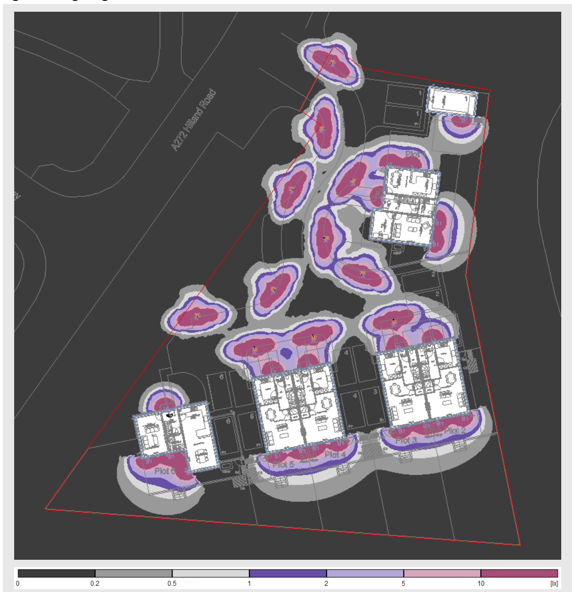
Figure 7.1 Lighting model false colour view - measurements in lux
