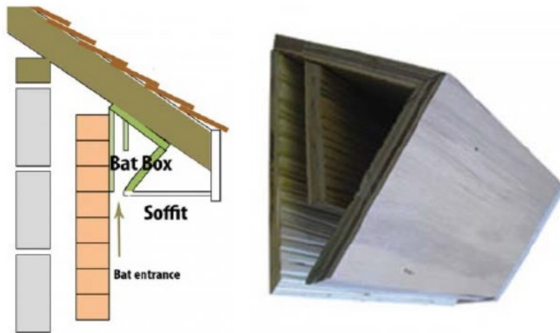
Figure 6: Soffit bat box (Wildcare)
