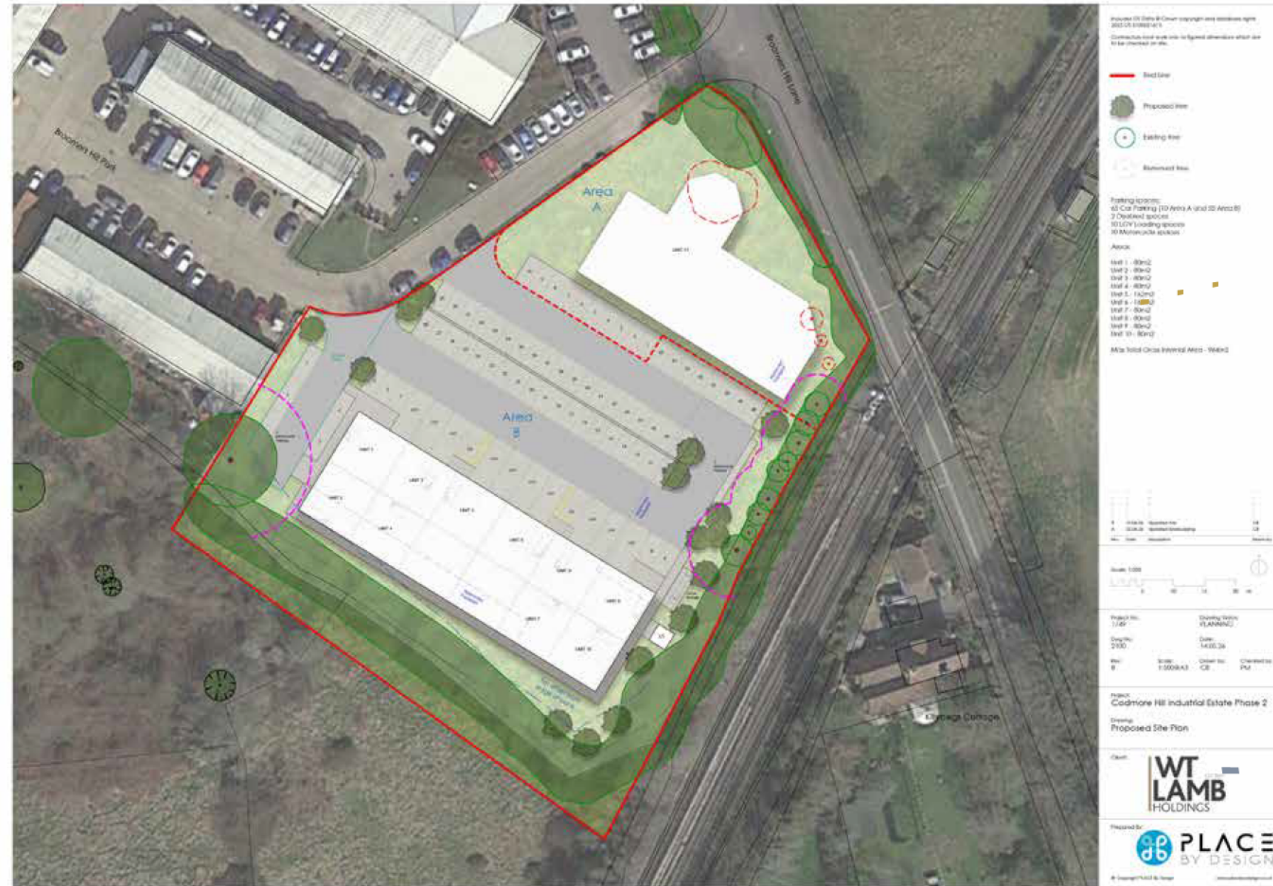
Figure 20 -Proposed site plan (Area B)
