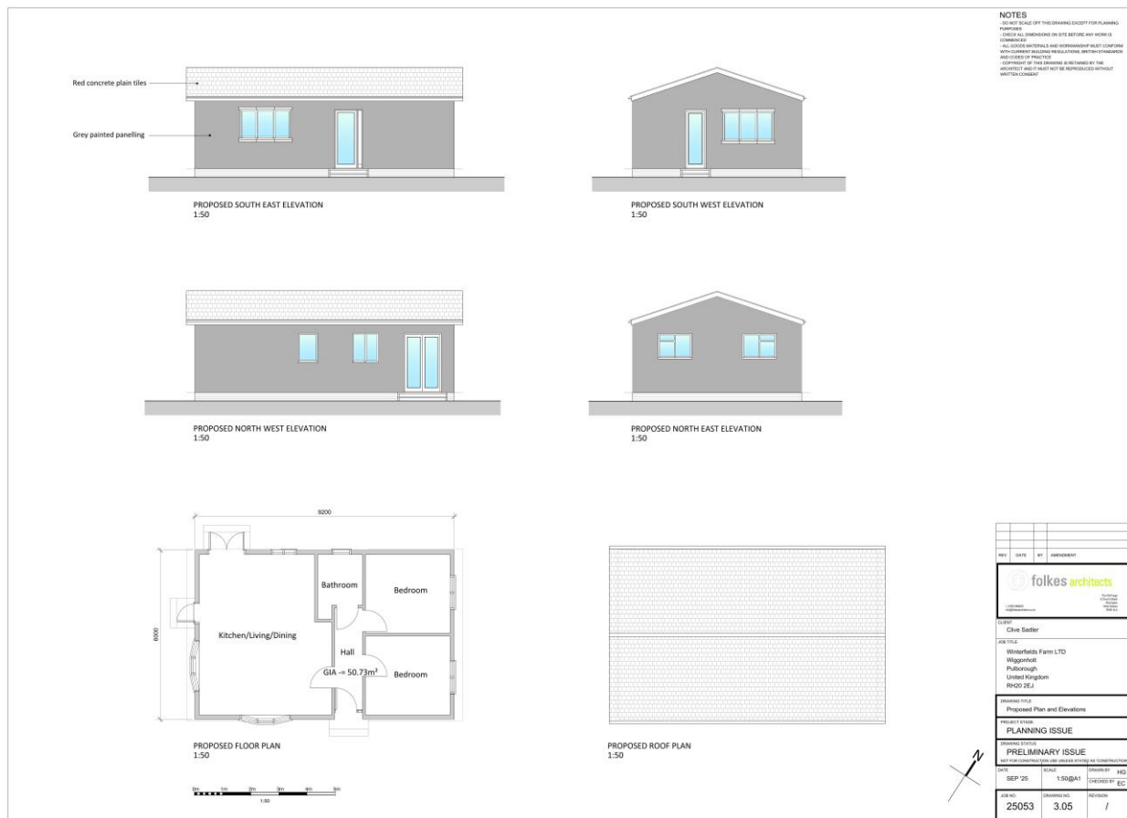
Figure A3. Proposed Plan and Elevations - Folkes Architects drawing 25053/3.05. The proposed unit is shown as approximately 9.2 m x 6.0 m.
