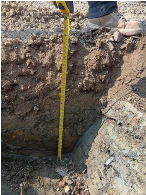
Inspection pit in Central Area on 6 th August 2025 showing subsoil to 250mm, with made ground underneath
