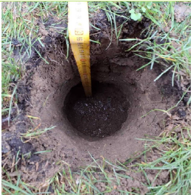
Inspection pit in Plot 1 area on 29 th January 2026 showing 600mm of clean cover including 350mm of Topsoil
