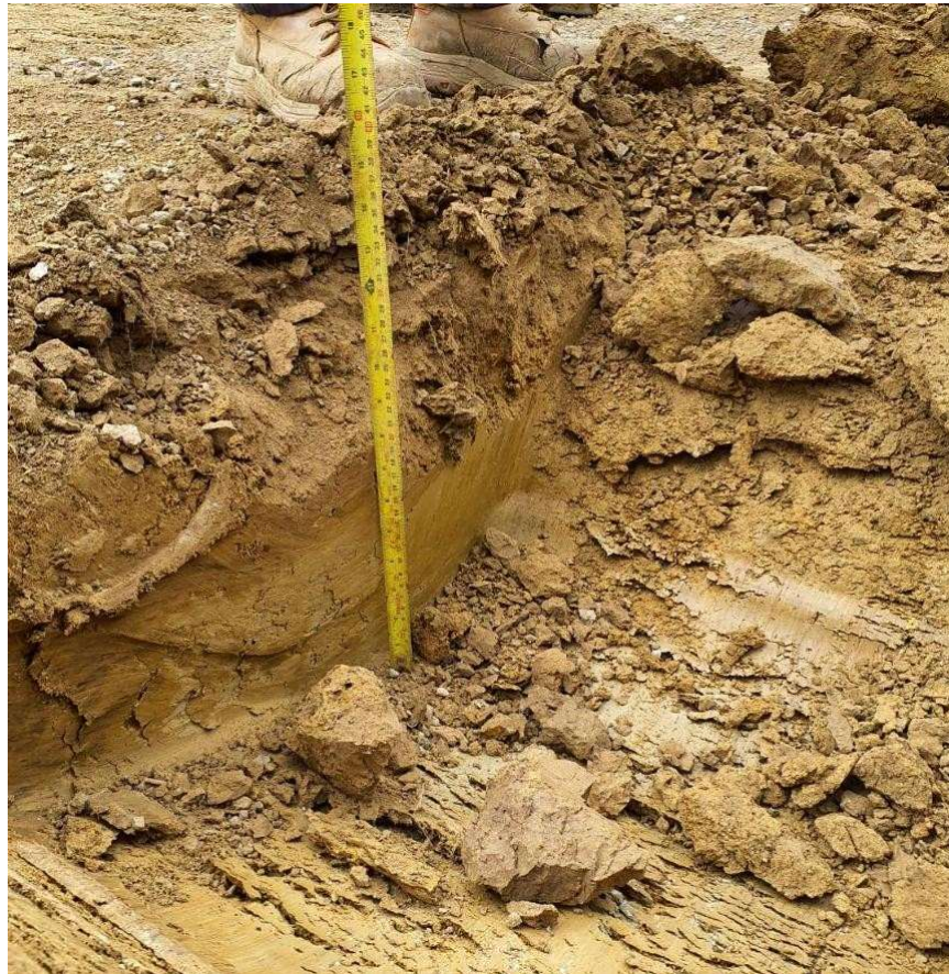
Inspection pit excavated 400mm in Plot 12
