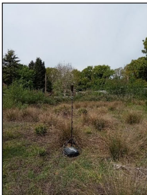
FIGURE 4.1: PHOTOGRAPH OF UNATTENDED NOISE MONITORING EQUIPMENT, N1
