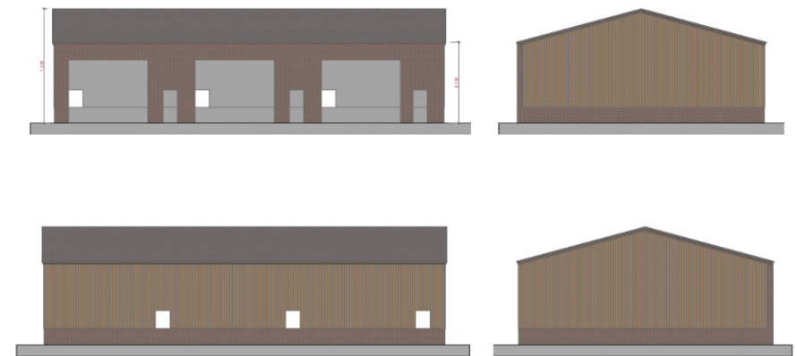
Figure 3.5 - Proposed Commercial Building Elevations
