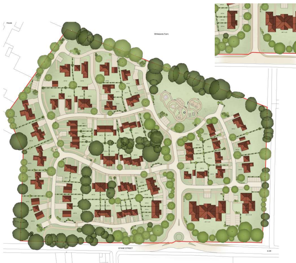
Fig. 10 – Extract of drawing no. 1726/SP-01, proposed site plan, Option 1 with an extract from drawing 1726-SP-02 depicting the alternative access (Option 2) inset.
