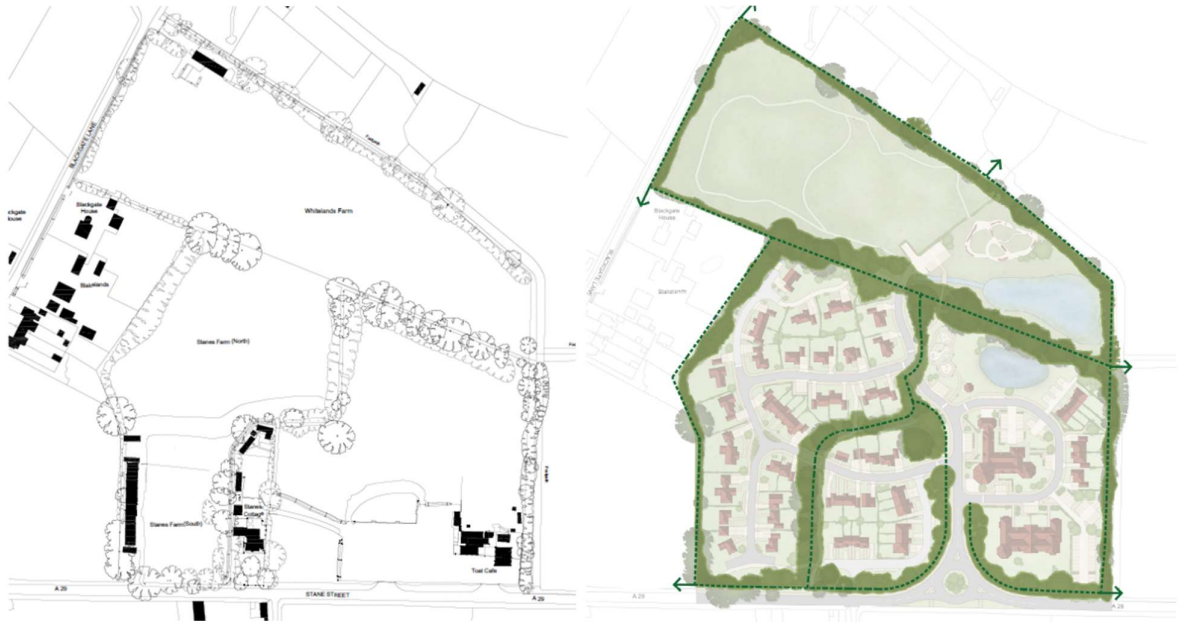
Fig 11 – Comparison of existing field boundaries on the existing site plan (left) with the proposal demonstrating their retention/enhancement (right)
