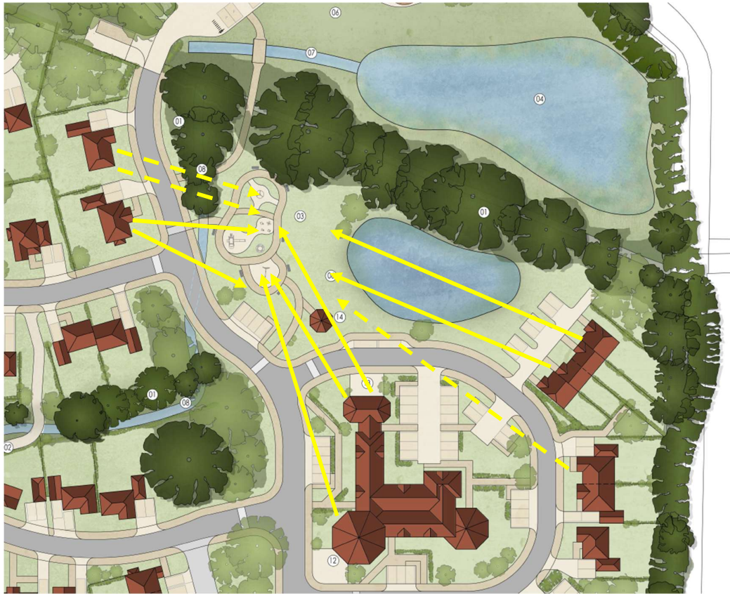
Fig 15 – Extract of the amended site plan drawing 1726/P-01 showing improved passive surveillance of public open space/LEAP area, illustrated with yellow arrows (shown dashed where views are filtered by vegetation)
