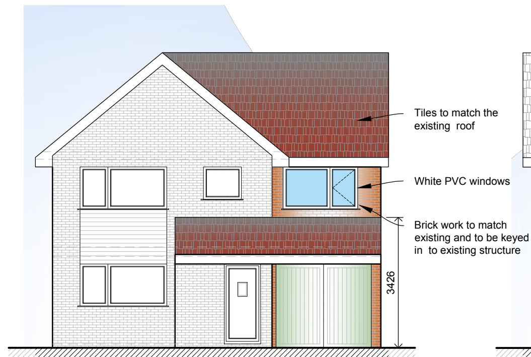
01 Front Elevation - As Proposed 3001 1:100 (at A3)
