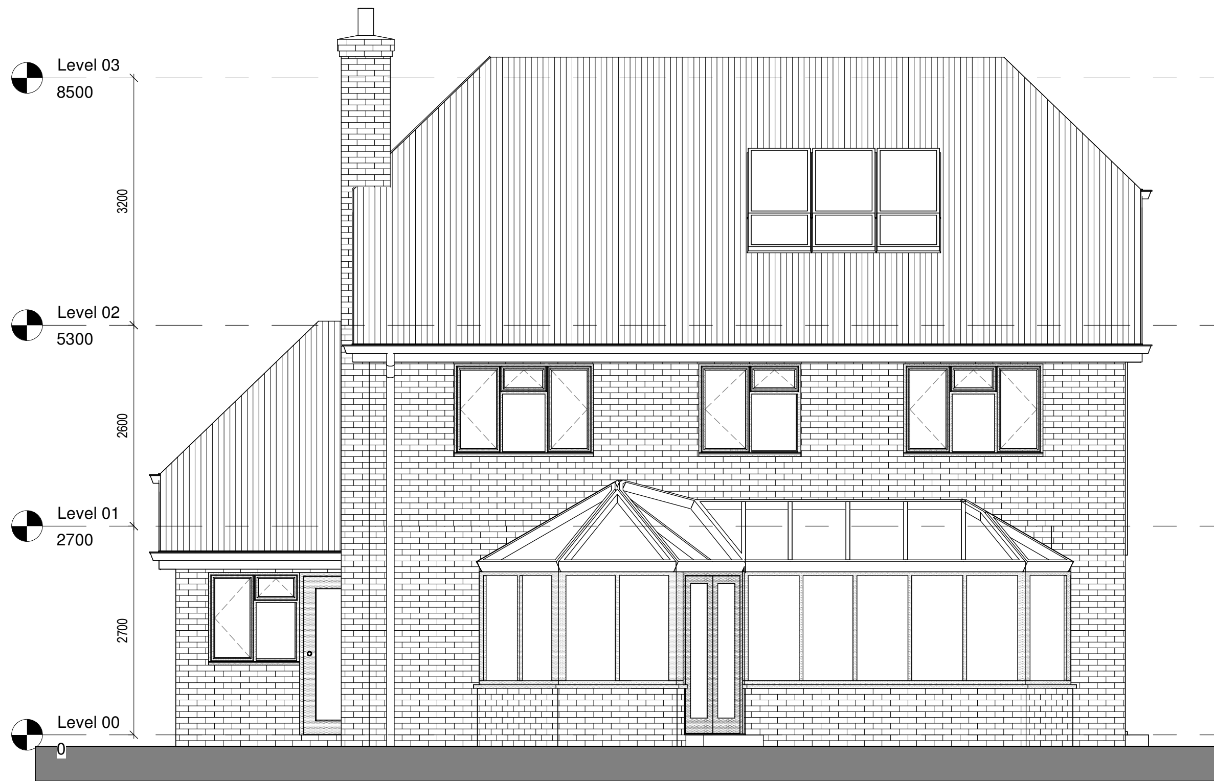
3 Rear Elevation - Existing 1 : 50
