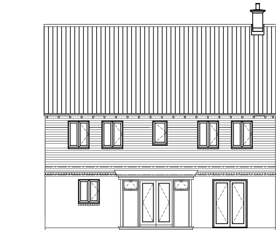
EXISTING REAR ELEVATION 1:100
