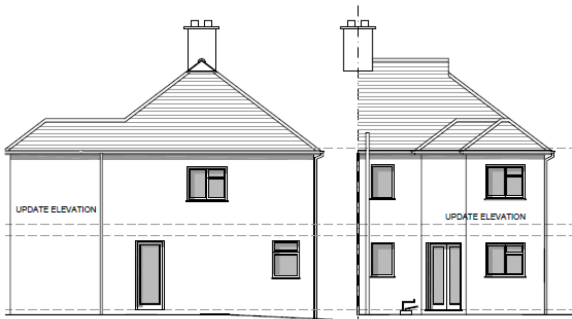
Fig 13. Proposed south elevation and rear (west) elevation
