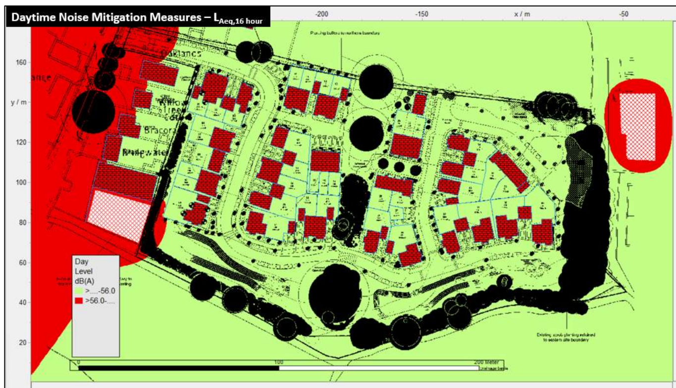
Figure 10. 2D Daytime Noise Mitigation Measures
