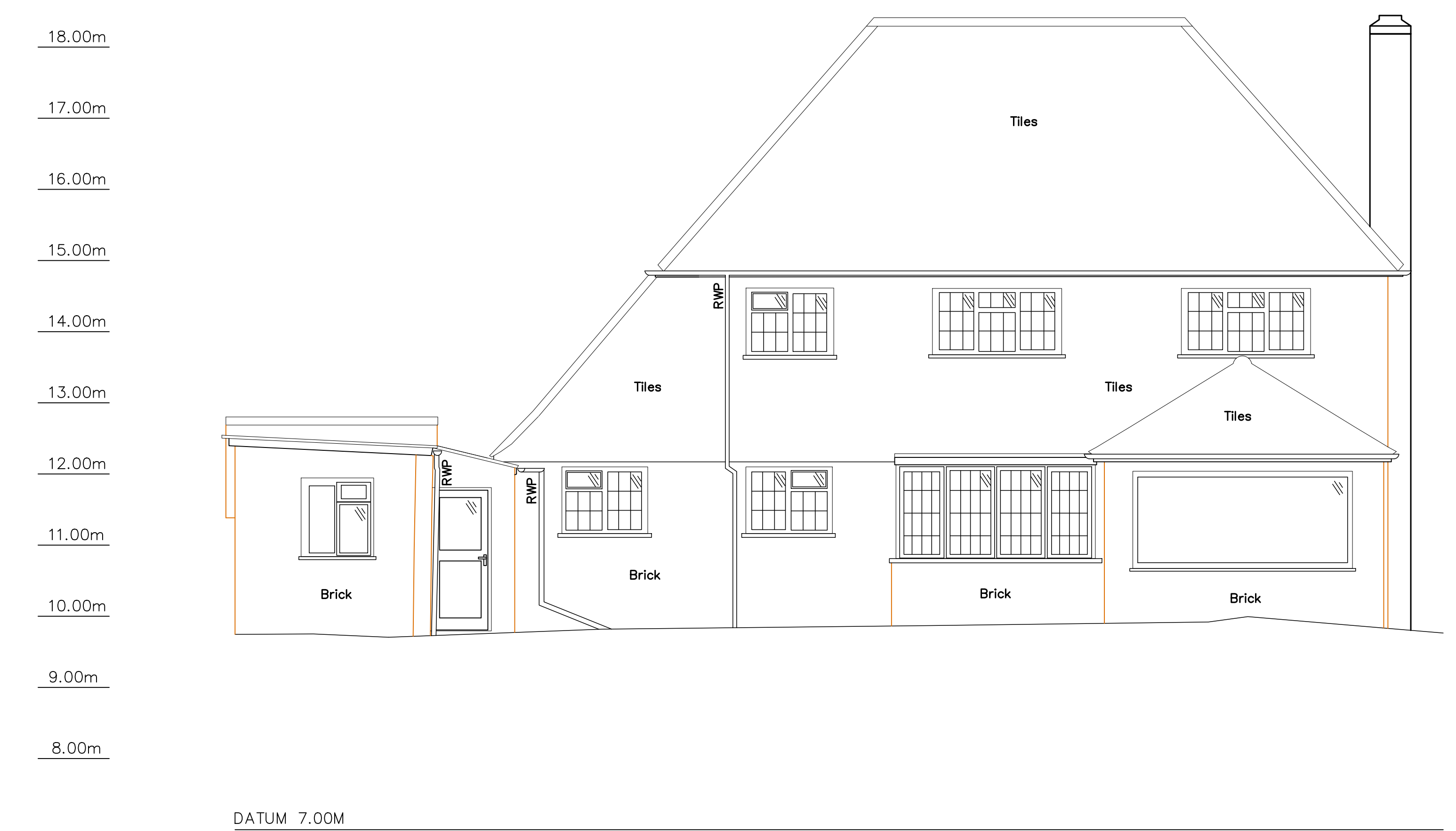
EXISTING SOUTH ELEVATION
