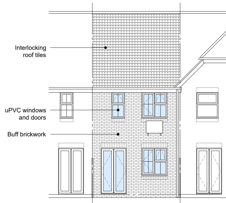
EXISTING REAR ELEVATION
