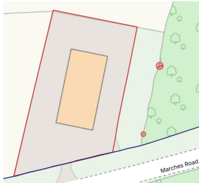
Figure 2 - Mark up received indicating the approximate locations of existing discharge points from the site into the watercourse, as confirmed by the site owner
