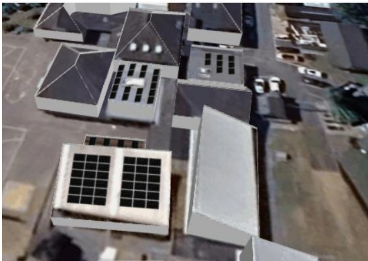
Figure 2: St Mary's C of E Primary School solar PV model output representation, looking west.
