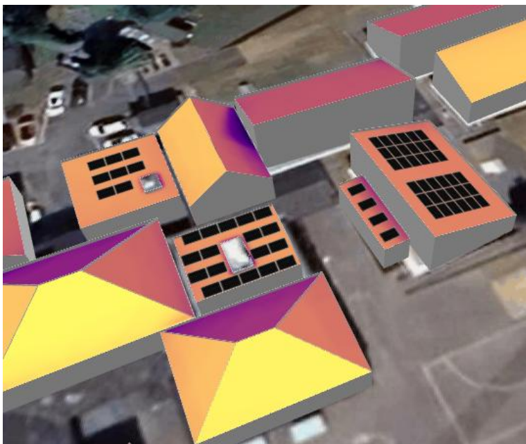
Figure 3: St Mary's C of E Primary School solar PV model irradiance representation, looking north.
