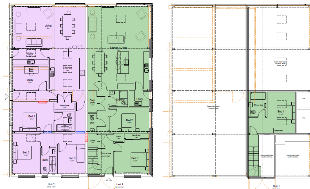
Figure 3.1 – Unit 1 & 2 Ground and First Floor Plans
