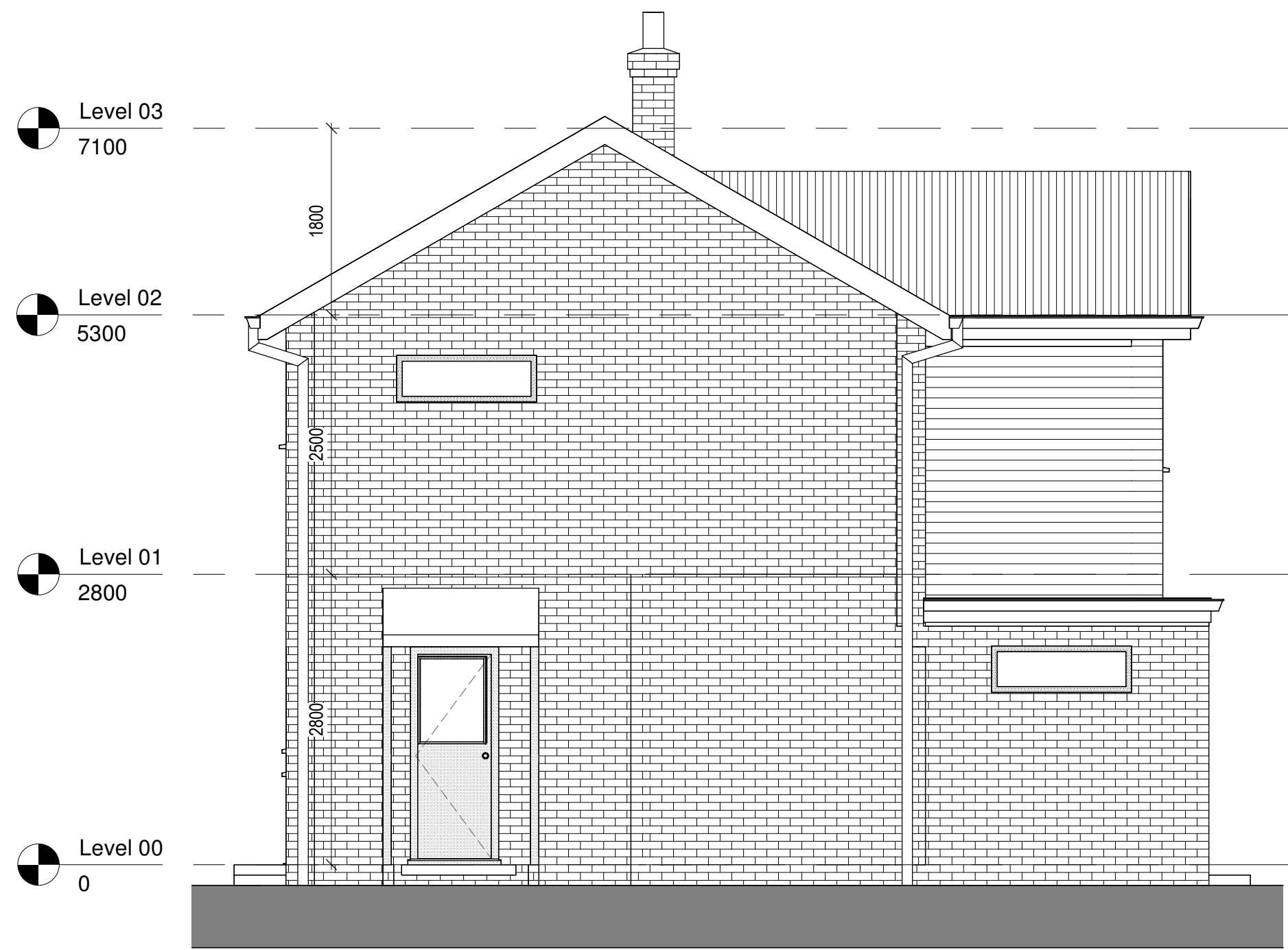
3 North Elevation - Existing 1 : 50
