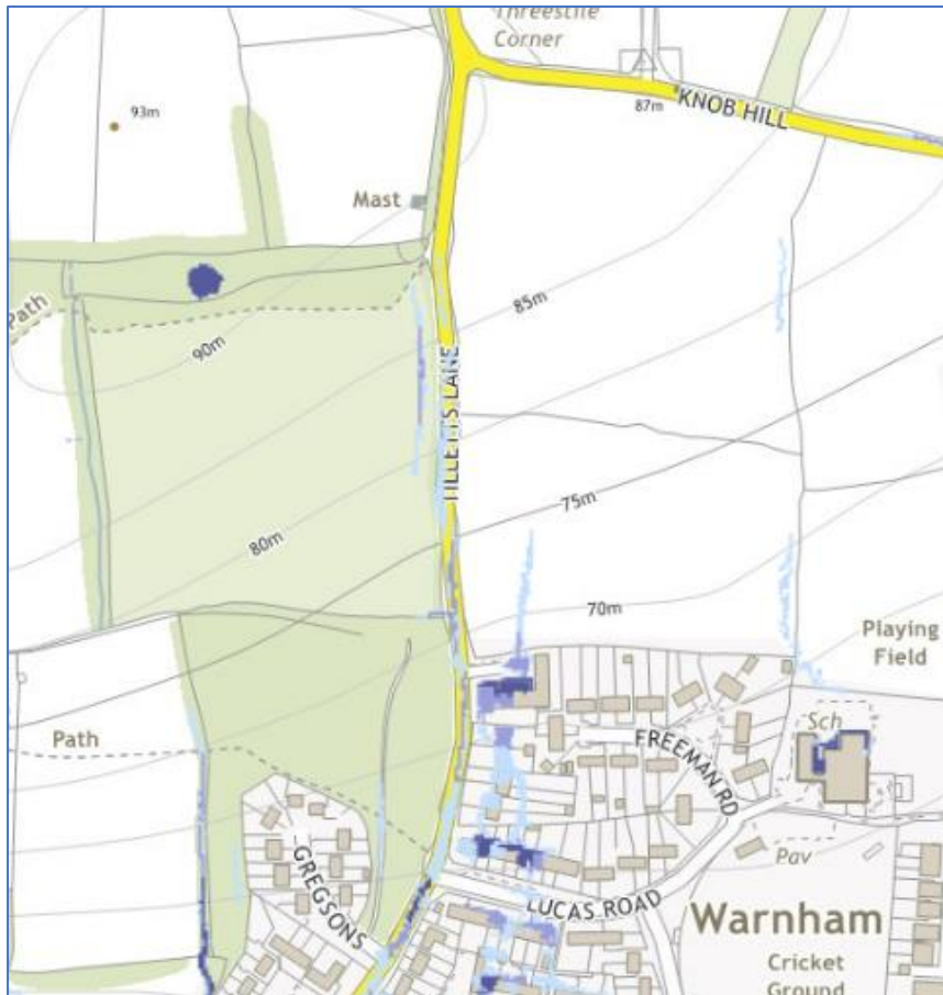
Image 2. Tilletts Lane area highway overlaid with surface water flood risk extents. Source: Ordnance survey mapping and Environment Agency surface water flood maps (extents). Accessed: 07/07/2025
