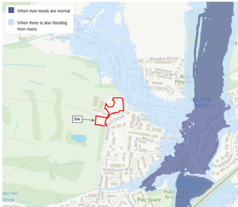
Figure 6.5 – EA Map of Risk of flooding from artificial sources showing the site at low risk of flooding.
