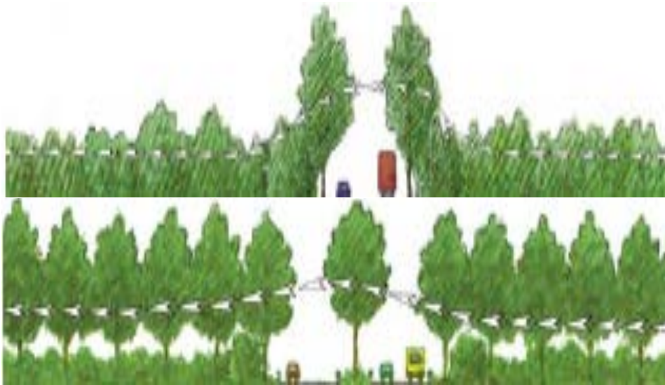
Figure 6: 'Hop-overs' created using trees to guide bats over roads (Limpens et al. 2005)
