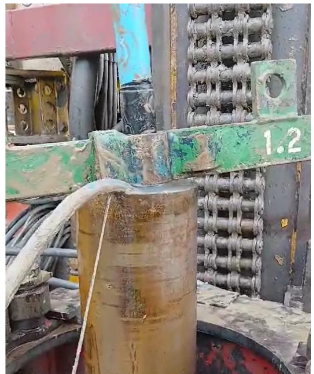
Figure 5-1 – Surface setup for drawdown testing
