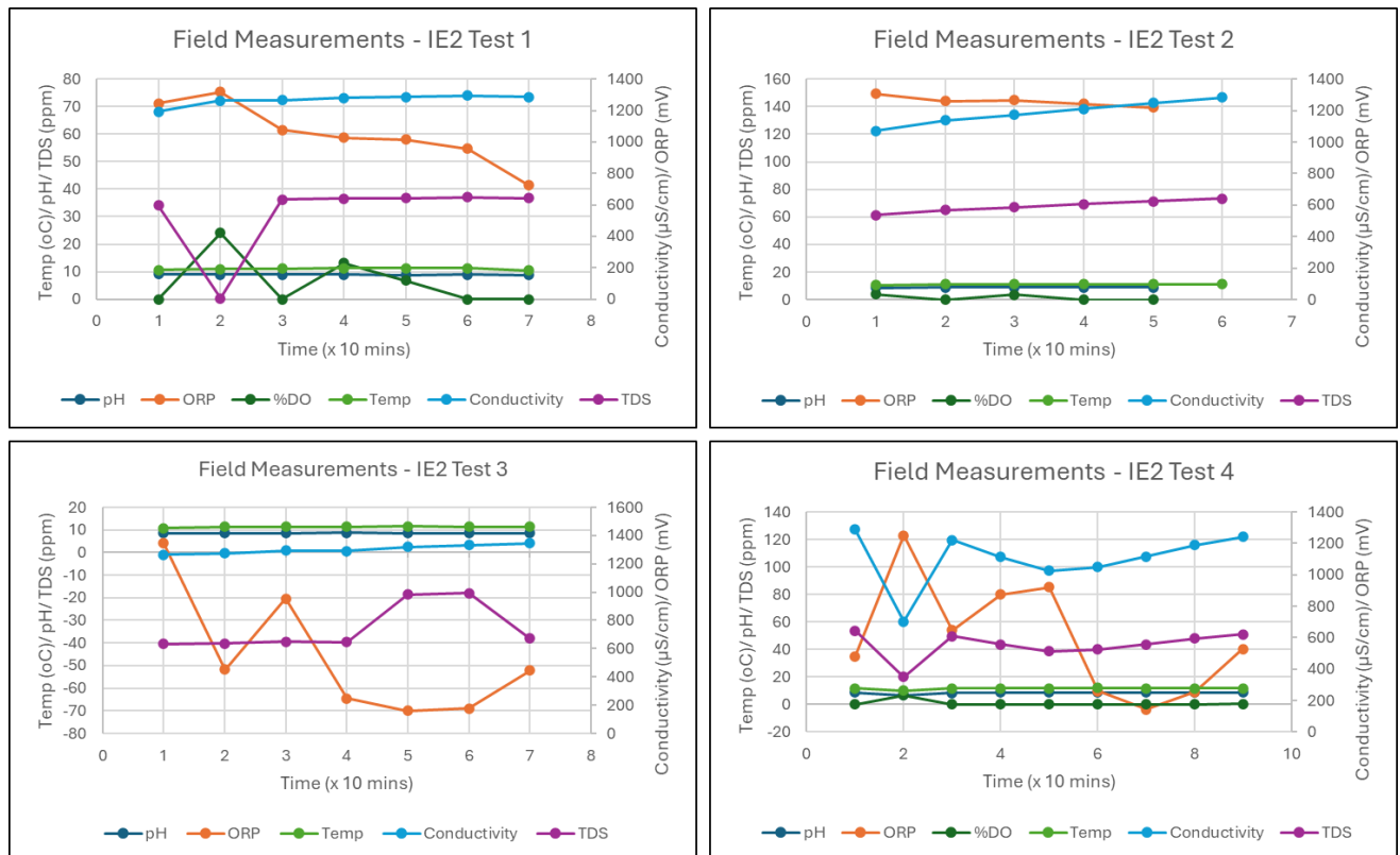
Figure 6.1 - Water temperature, ORP, electrical conductivity, pH, TDS and DO concentrations measured at the well head during pumping tests at borehole IE2
