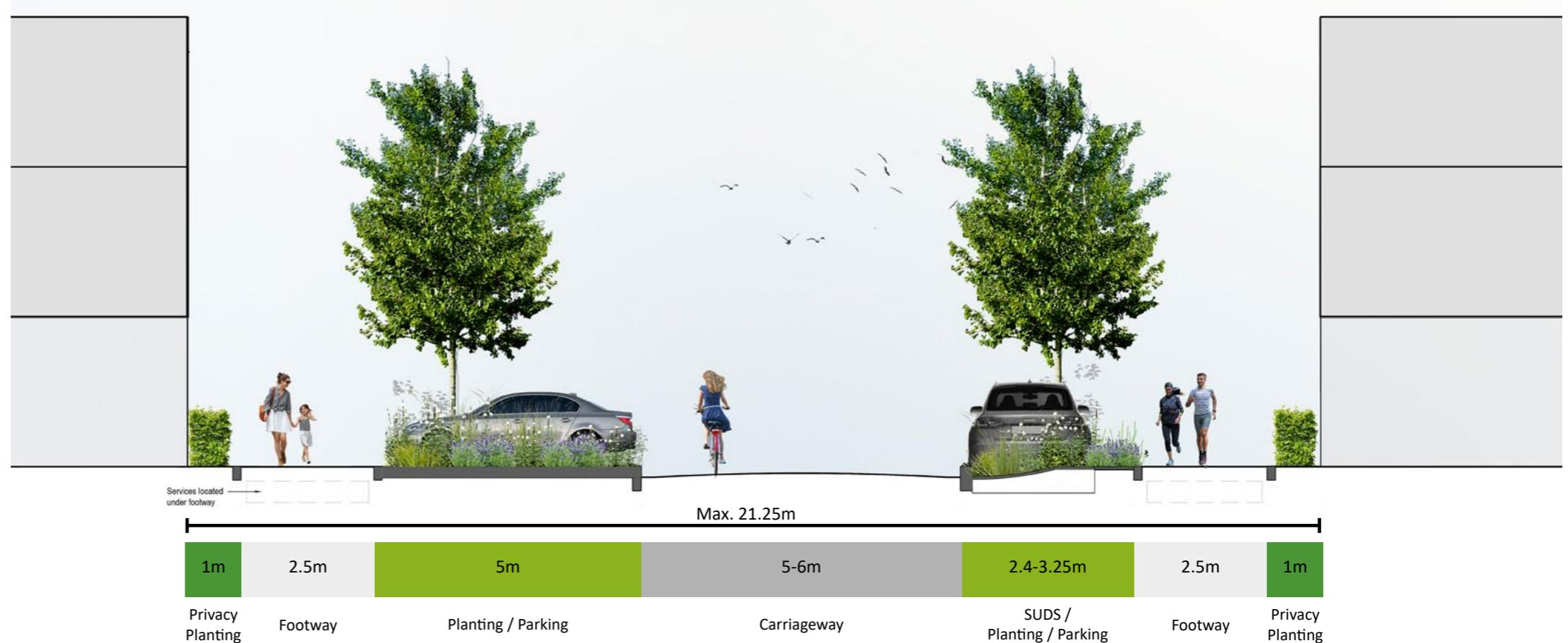
FIGURE 28 Secondary street arrangement
