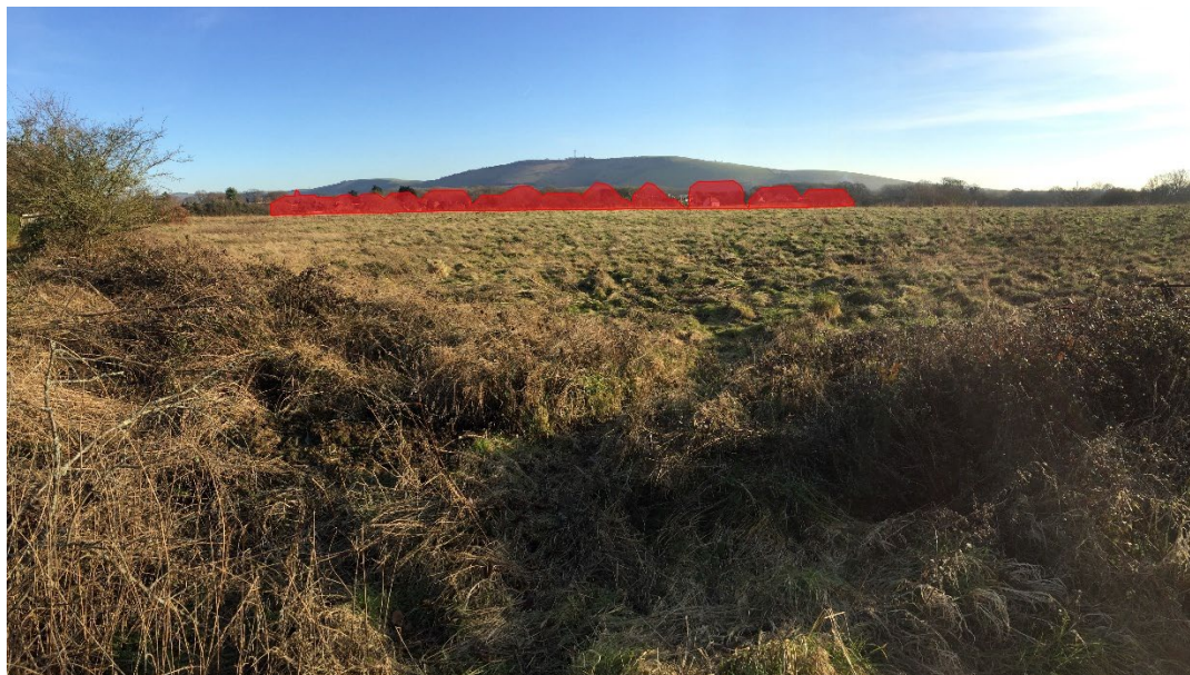
Figure 1: Type 2 Illustrative Photo-wireline from the elevated ground within the site. This image combines a photograph (taken from the north-western corner of the site in winter 2023) with an accurate computer model of the proposed development, using existing houses, landforms and vegetation as reference points.
