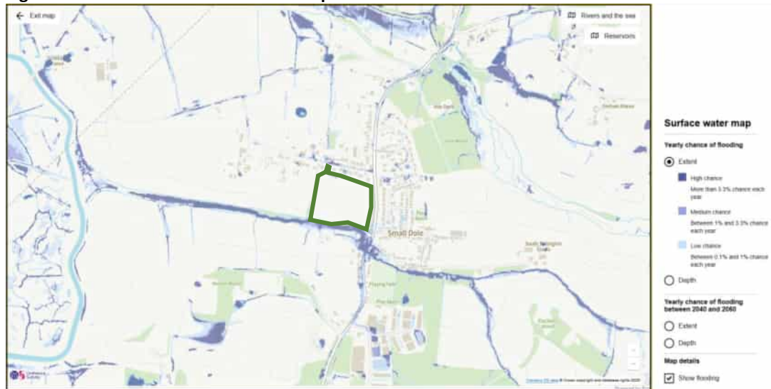
Figure 4.3: Surface Water Flood Risk Map
