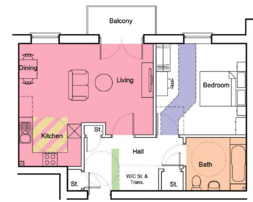
Example floor plan of proposed M4(3) compliant apartment.
