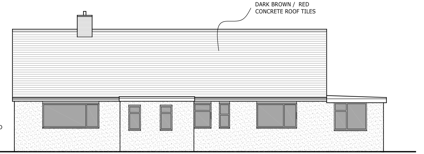
EXISTING REAR ELEVATION 1:100@A1
