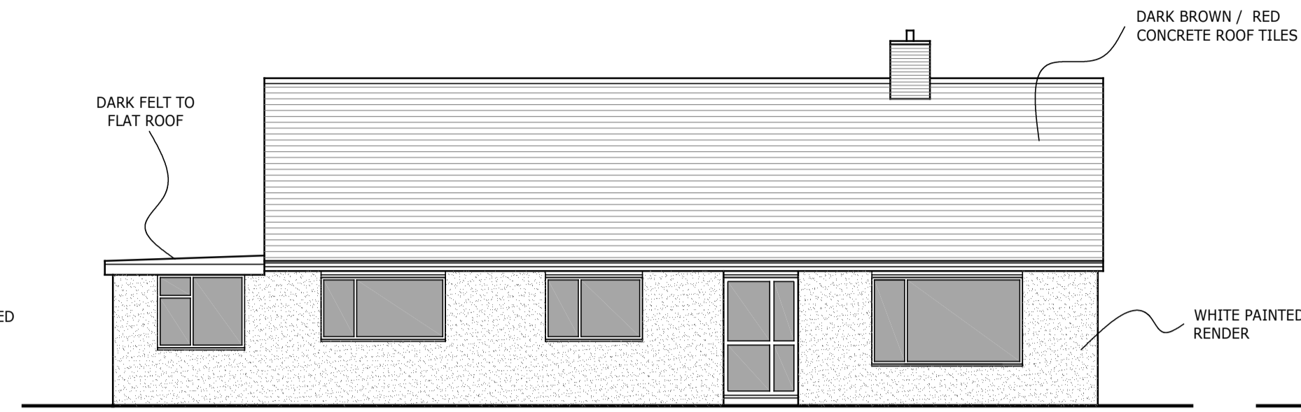
EXISTING FRONT ELEVATION 1:100@A1
