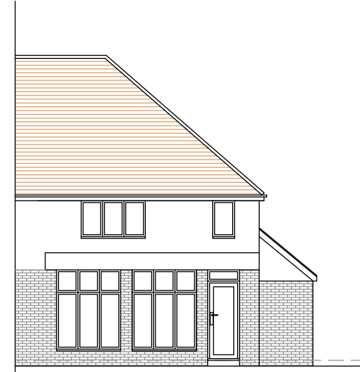
Existing Front Elevation (East), Scale 1:100
