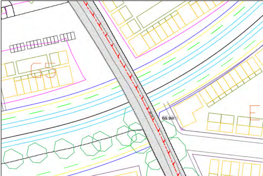
Figure 21: Thames Water Assets Overlaid with Development Proposals – Intersection of Proposed Phase 1B Crawley Western Link Road and Existing Rusper Road
