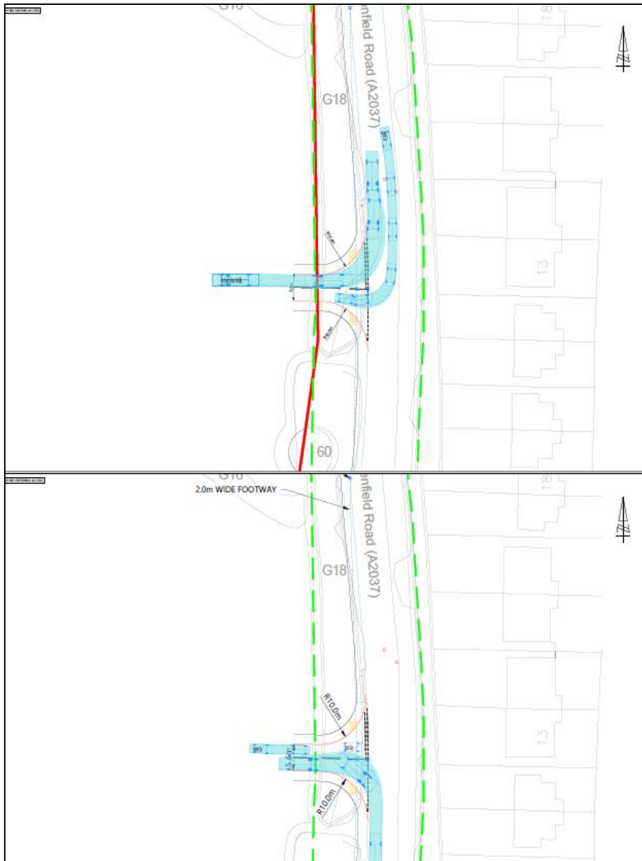
Image 2.2: Swept Path Analysis – Refuse Vehicle and Large Car
