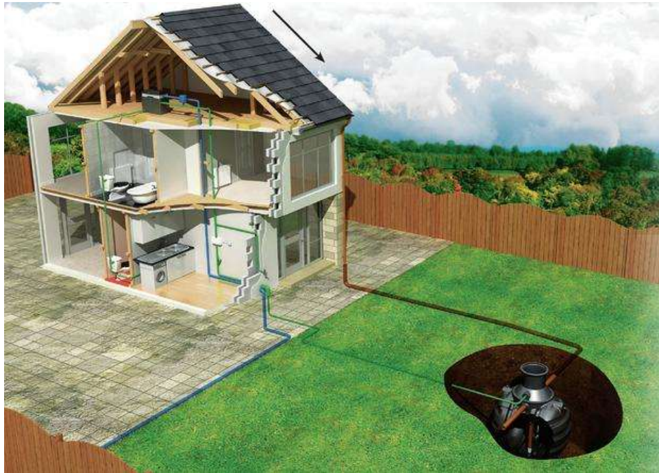
Figure 7: Schematic of domestic rainwater harvesting system
