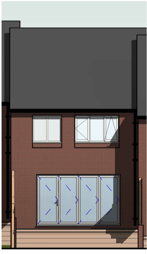
Proposed Rear Elevation 1 : 100
