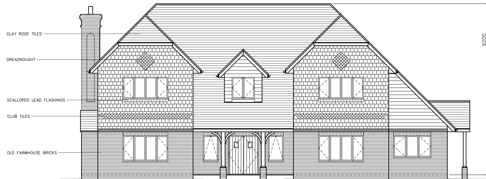
FRONT ( West facing ) ELEVATION
