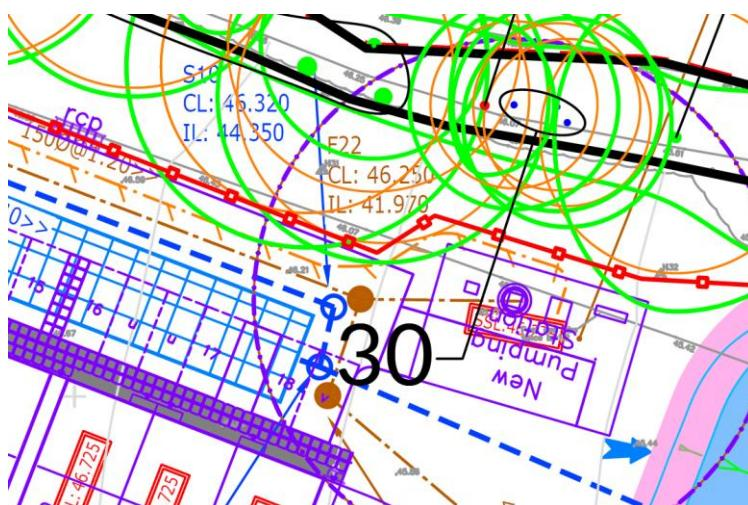
Drainage routes to the pumping station are outside the root protection area and can be implemented conventionally and not result in harm to the trees.
