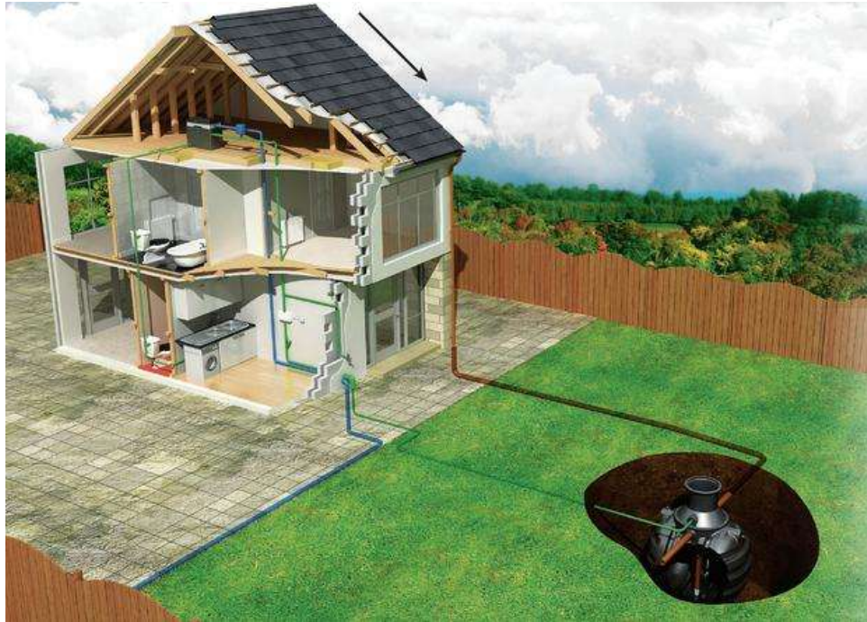
Figure 7: Schematic of domestic rainwater harvesting system
