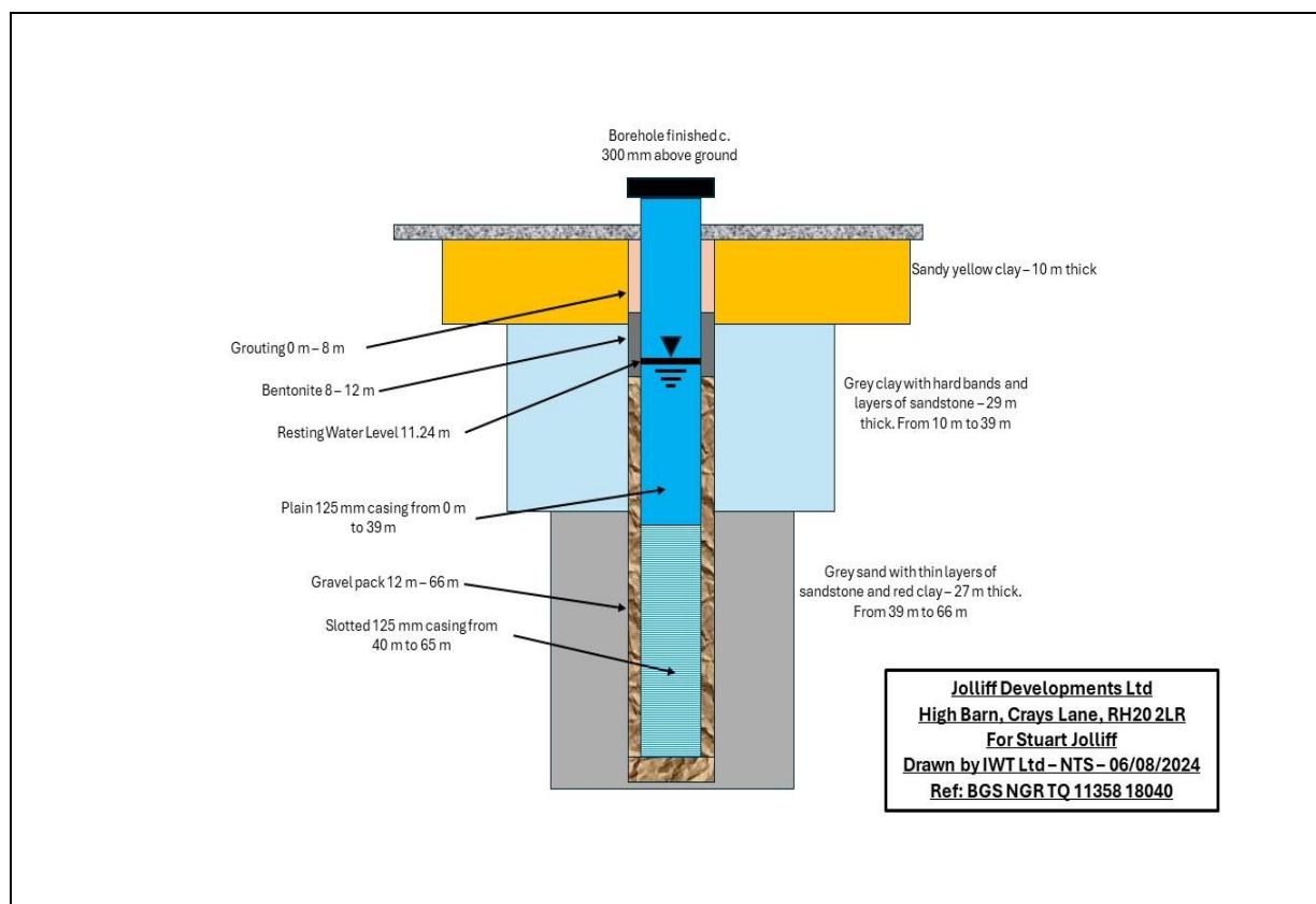
The borehole has been drilled as per the drill log attached to the email and as below (page 1 of log). The borehole produces water from the grey sands/sandstone and red clay. The borehole has been finished above ground. There are no known sewage systems or ground contamination sources nearby.
