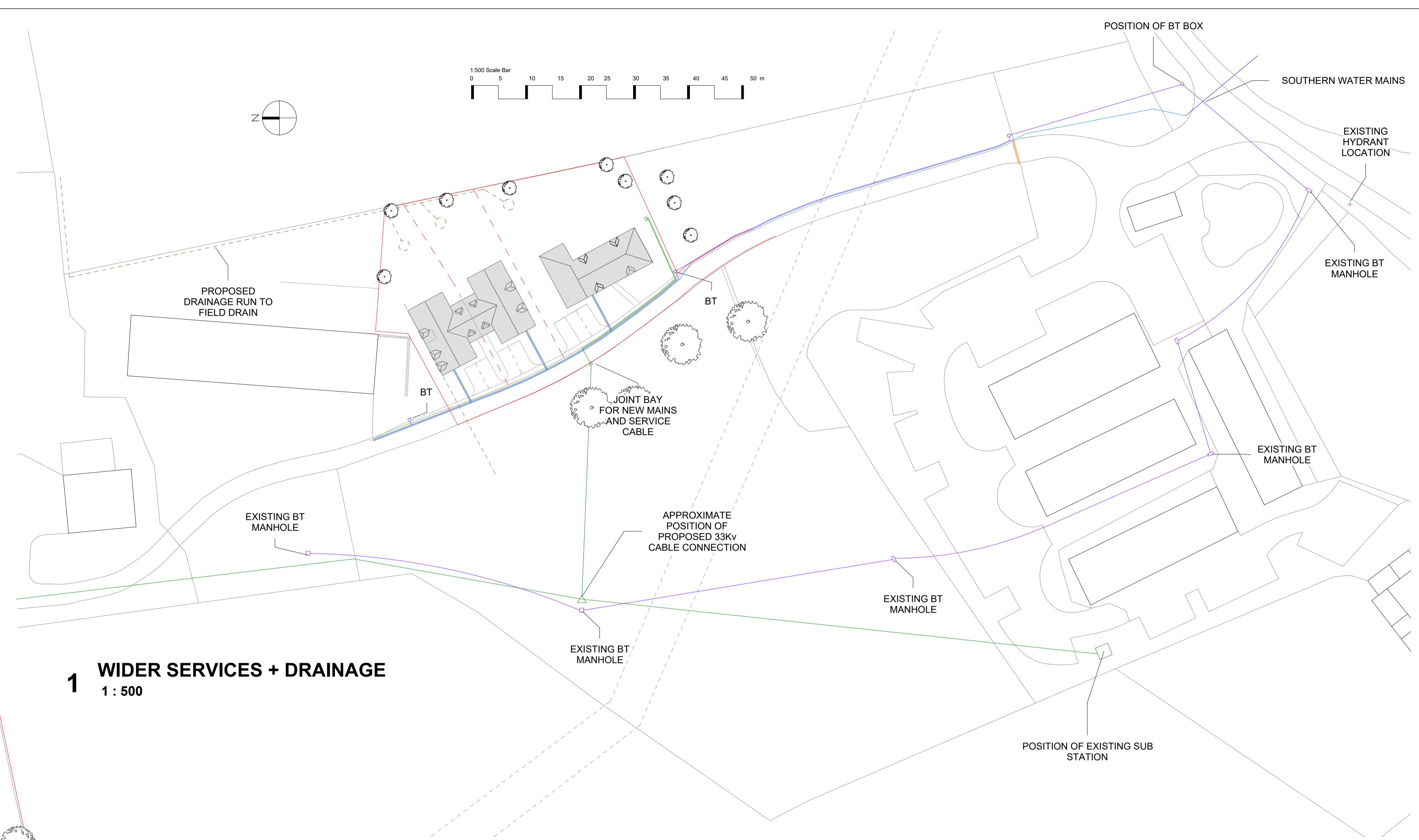
WATER - CONNECTIONS TO BE TAKEN THROUGH THE GATE AREA TO KEEP THE SUPPLY RUNNING ALONGSIDE THE DRIVEWAY TO THE FRONT OF THE HOUSES. POTENTIAL HYDRANT REQUIRED.
