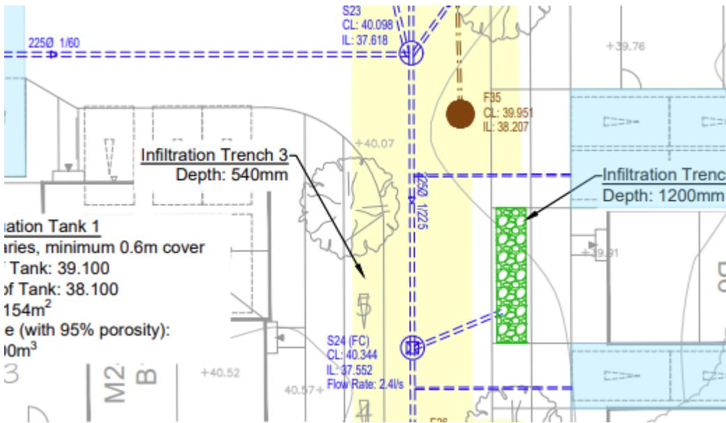
The depths of the infiltration trench's in the calculations needs to match the drainage layout. For example, trench 2 has a depth of 1775mm in the modelling calculations, but 1100mm in the drainage layout.
