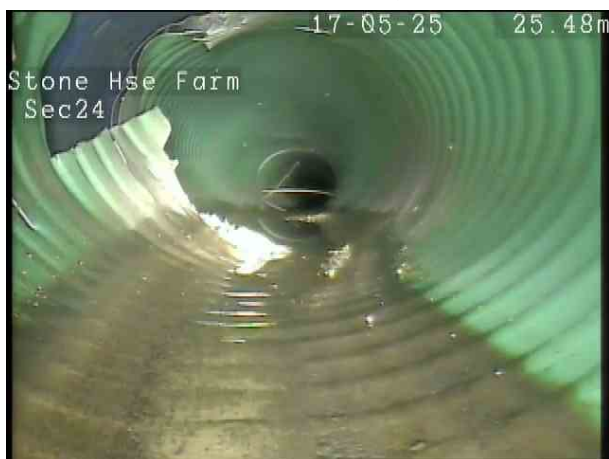
2a506dbd-b296-473b-aea1-4d9dfa2912e9.png, 00:03:32, 25.50 m Deformed sewer or drain, 25%
