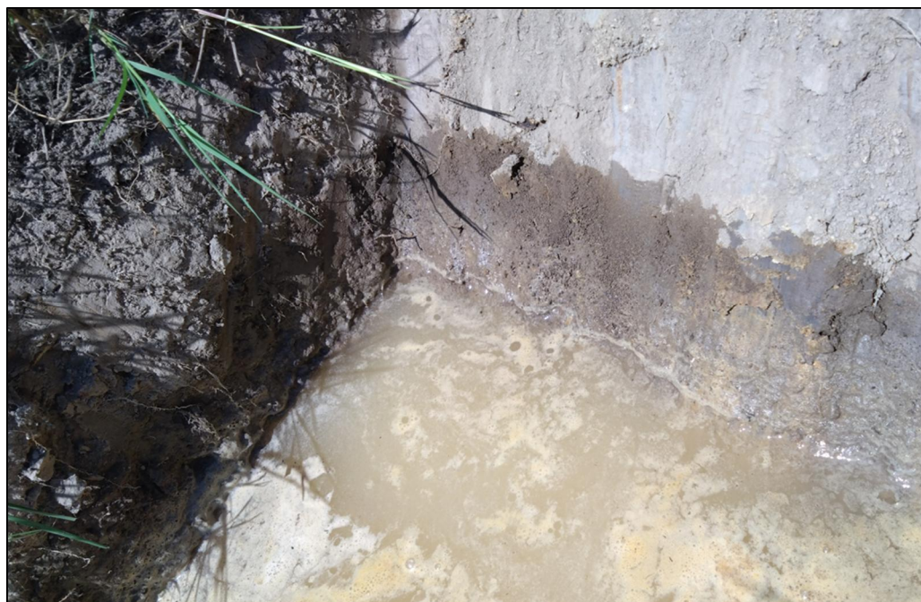
Figure 2.3 – Upward Capillary Absorption of Water Into Dry Topsoil
