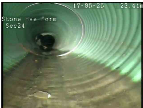
bcf0778e-dc5c-47ea-8fdd-651319b08627.png, 00:03:10, 23.50 m Deformed sewer or drain, 20%
