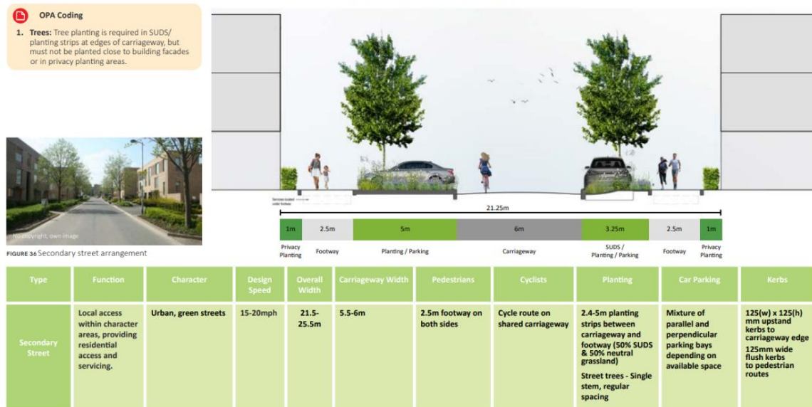
Figure 4.4: Typical cross section for Secondary Streets (Design Guide).
