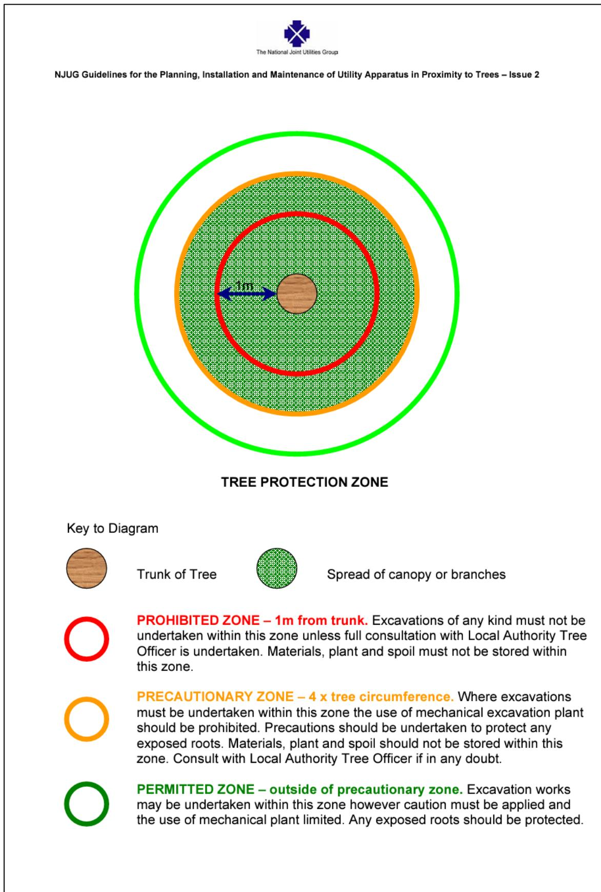
Figure 6: additional guidance on working close to trees (The National Joint Utilities Group, 2007).
