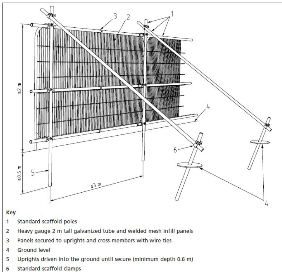
5.3.7 The default specification comprises a scaffold framework onto which 2m tall, welded mesh panels such as 'heras' panels will be secured to uprights and crossmembers with suitable anti-tamper couplers. The scaffold framework will be driven into the ground to a minimum depth of 600mm below existing ground levels, ensuring that care is taken to avoid damage to existing roots.
