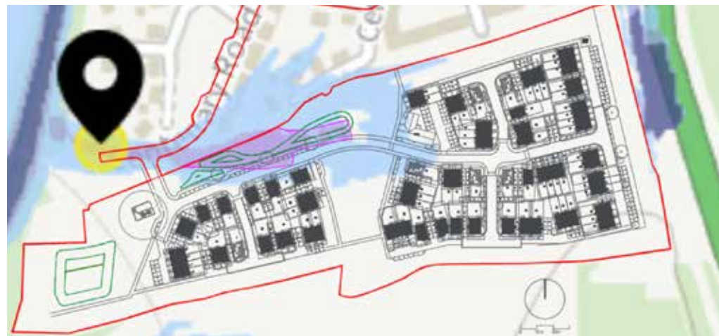
Figure 4. Layout with flood mapping & proposed drainage features as per pre-application & initial application submission
