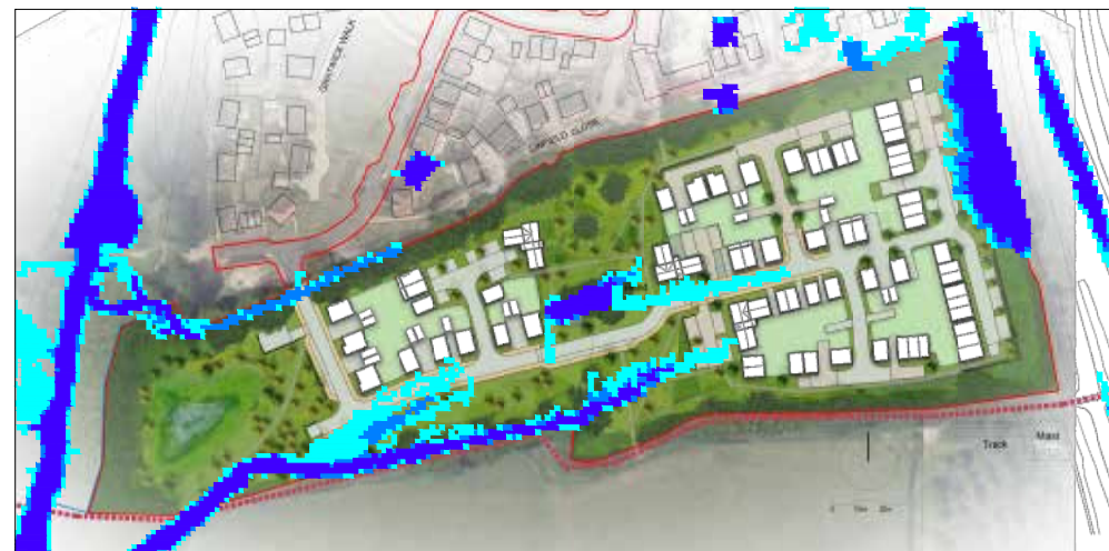
Figure 8. Revised layout with flood mapping and proposed drainage features
