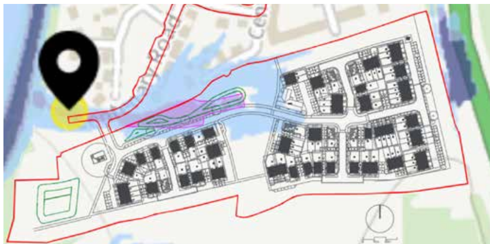
Figure 7. Initial layout with flood mapping and proposed drainage features
