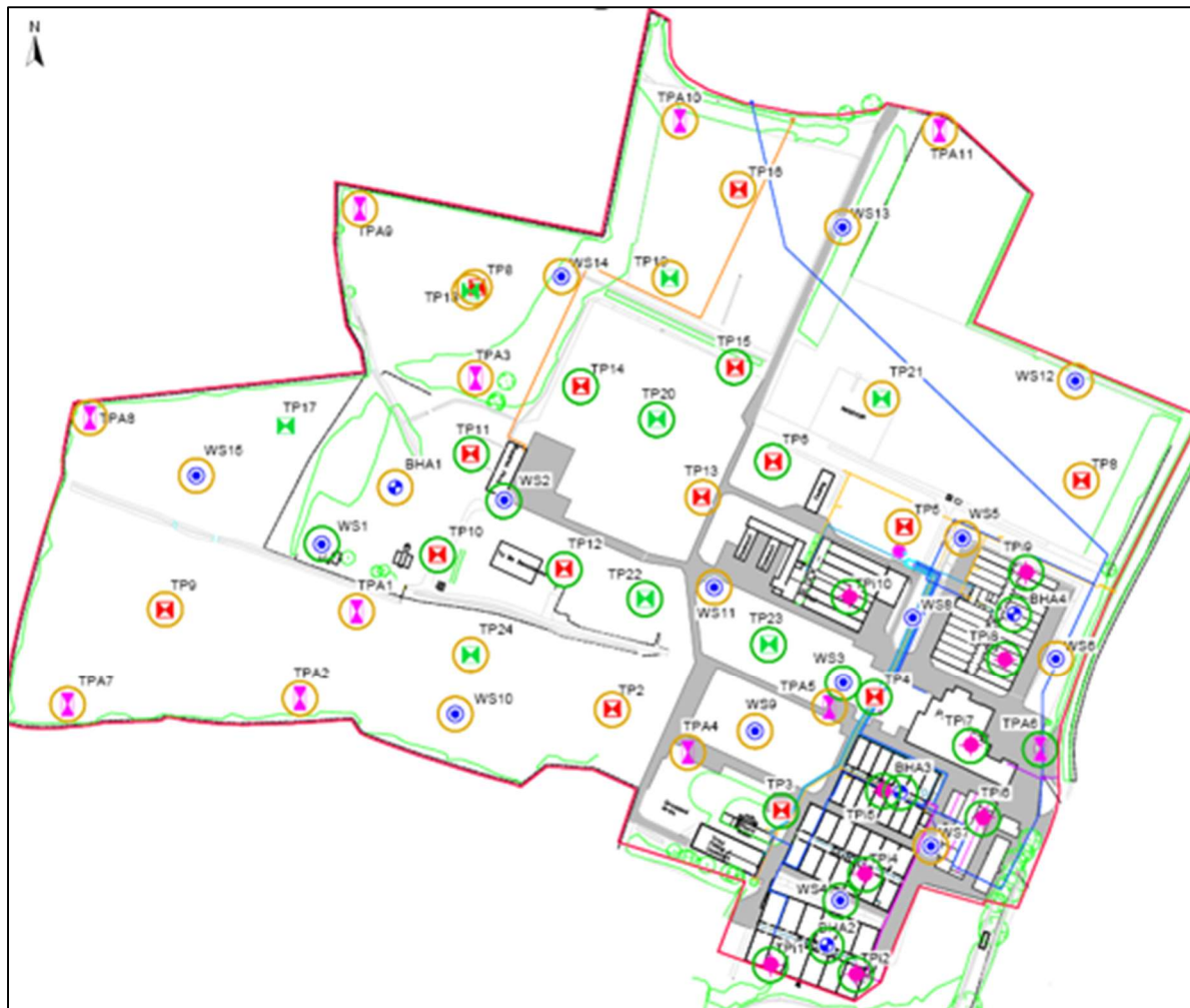
Figure 3-4: Exploratory Hole Location Plan (Source: RSK Geosciences)
