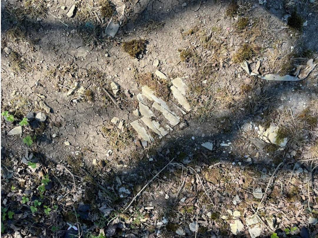
Photo 8 – Fragments of suspected asbestos cement on the ground surface.
