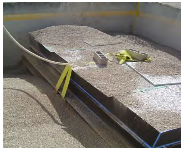
Filling the test pit with gravel and simultaneously filling the plant with water
