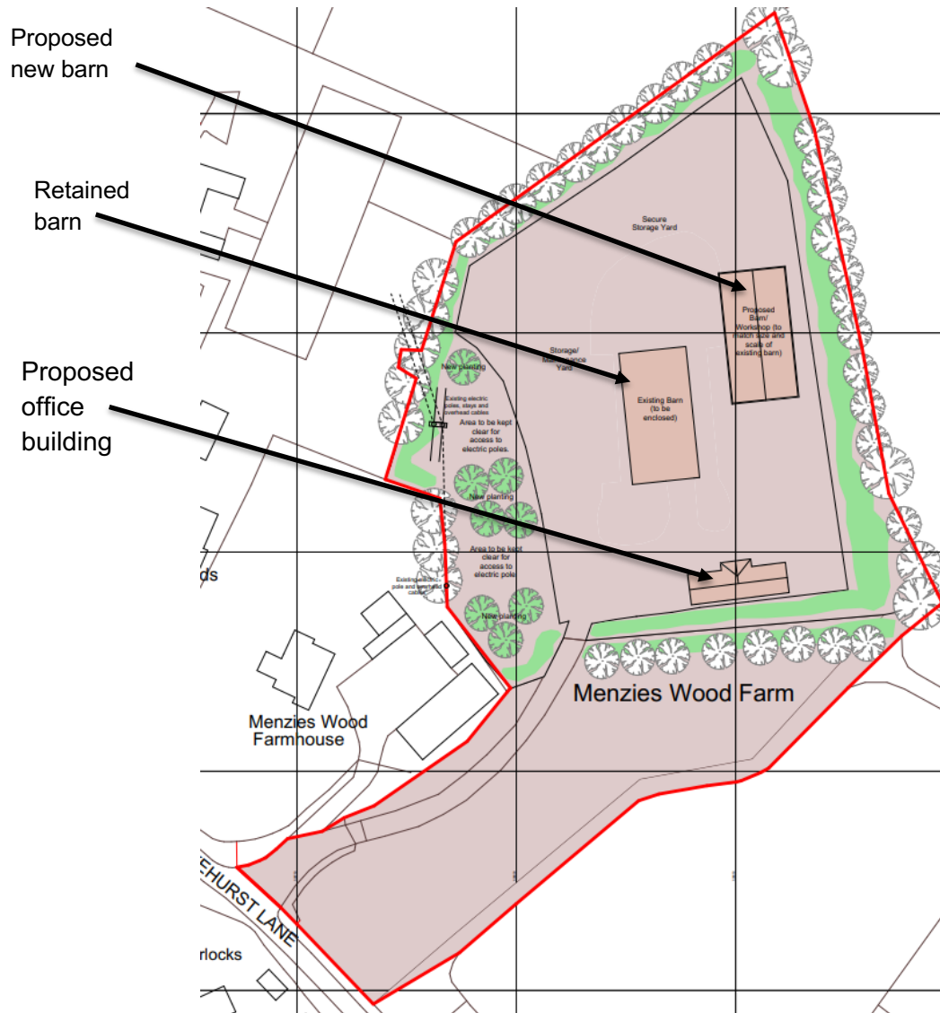
Figure 3.1 - Proposed Block Plan
