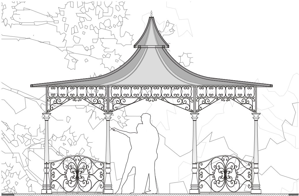
Proposed detailed elevation showing the intricate metalwork
