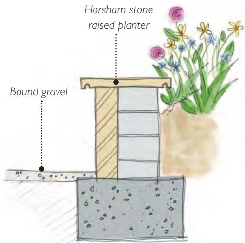
Typical section of Horsham stone raised planter retaining wall
